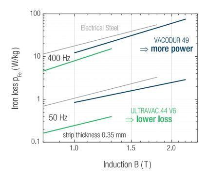
In comparison to Electrical Steel VAC alloys offer lower iron losses in all cases:
