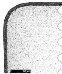
Fig. 11: Micrograph of edge coverage with VACCOAT
